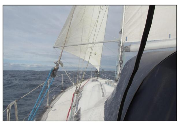
After day break I found the answer to the puzzle of what had caused the port staysail sheet to chafe. With the sail in its normal position the sheet ran inside the stays clear of all obstructions. Once the jib was poled out the block on the track leaned outward and the sheet was rubbing hard on the lower part of the inner side stay. We realised that the sheet should be threaded outside the stays aft to the next turning block when the staysail was poled to windward and did that.
